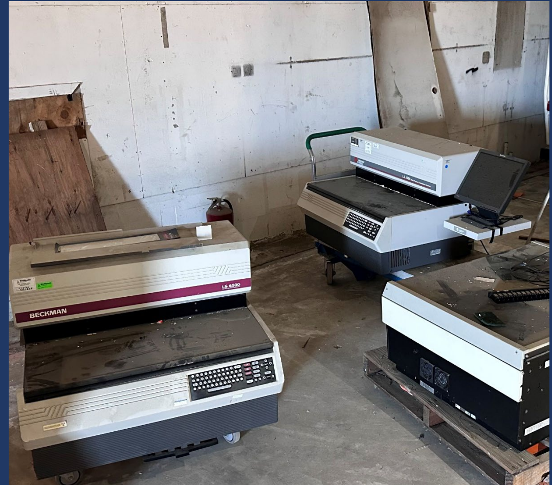
Liquid scintillators are specialized laboratory instruments used for radiological analysis
